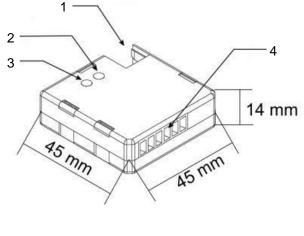
1. KNX bus2. LED3. Programming button4. Socket
