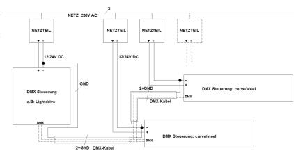
**IMPORTANT:** To ensure correct functioning of the DMX bus when using several voltage sources, the negative pole of the power supply and the actuator must be connected together with the GND of the DMX, to avoid a shift of potential.
