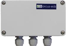
SK08-AN2 |         | <p>KNX Dataconverter / controller for monitoring and control of two analog voltages.<br/>Input range 0 .. 12 VDC.</p> <p>Plastic housing: 115 x 65 x 55 mm<br/>IP54/65</p> | 30806202    |
