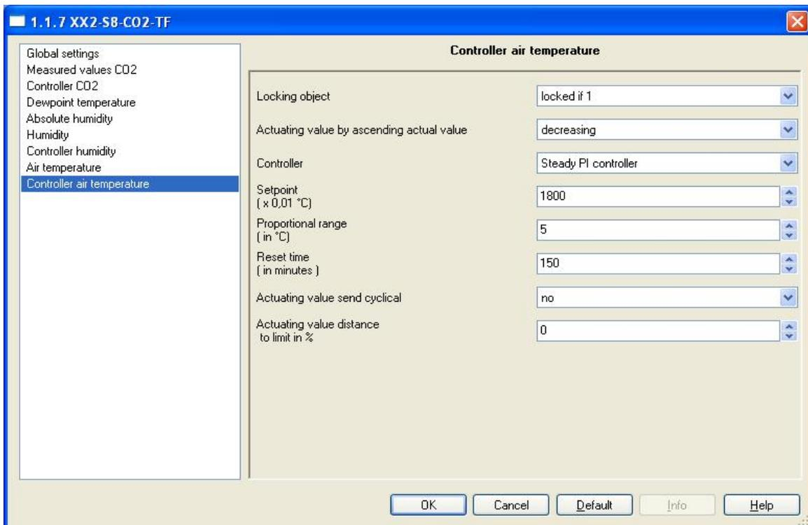
The settings for the air temperature controller are analogue for the measured value CO2. The rates for set points, differential gap and proportions should be done in steps of 0,01°.
