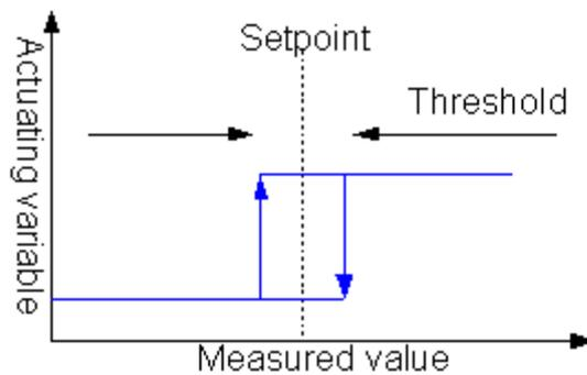
**Two-Position Control with Pulsed Output:**
