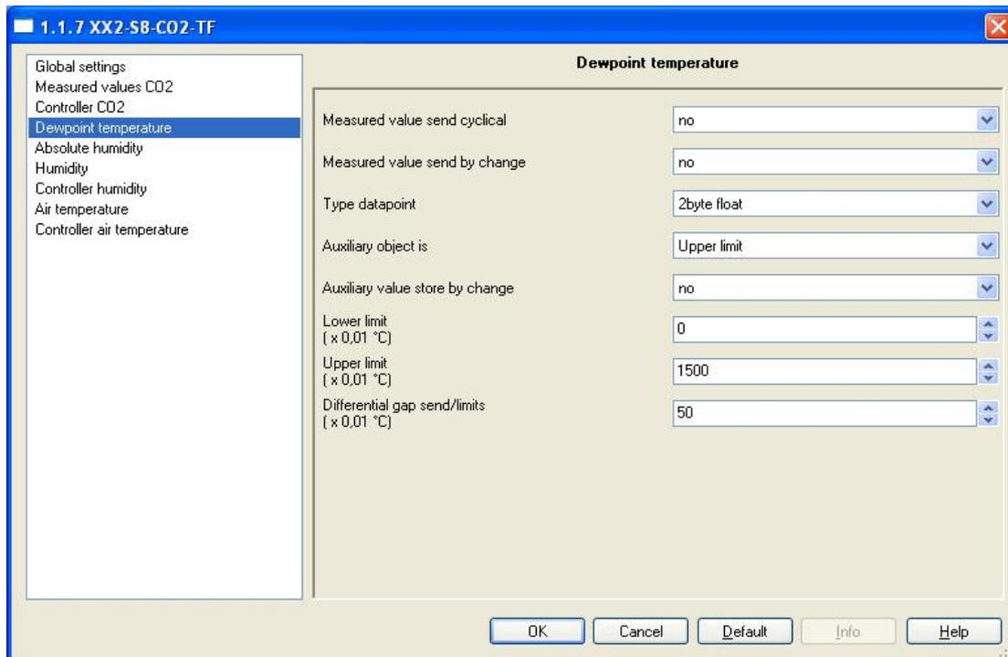
The settings for the arithmetic value of the dew point temperature are analogue for the measured value of CO2. The rates for thresholds and hysteresis should be done in steps of 0,01°.
