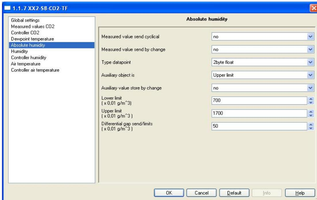
The settings for the arithmetic value of the absolute humidity are analogue for the measured value of CO2. The rates for thresholds and hysteresis should be done in steps of 0,01 g/m<sup>3</sup>.
