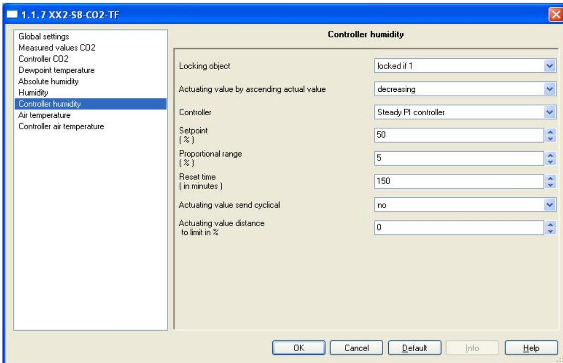
The settings for the relative humidity controller are analogue for the CO2 controller. The rates for set points, differential gap and proportions should be done in steps of 1%.
