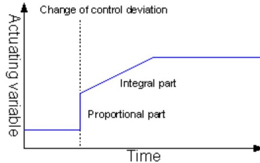
**Continuous PI Control with Pulsed Output (PWM):**
