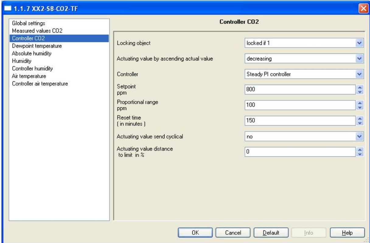
**Controlled Variable with increasing actual value: decrease/increase** The Actuating direction of the controller can be adapted to the characteristics of the controlled system.
