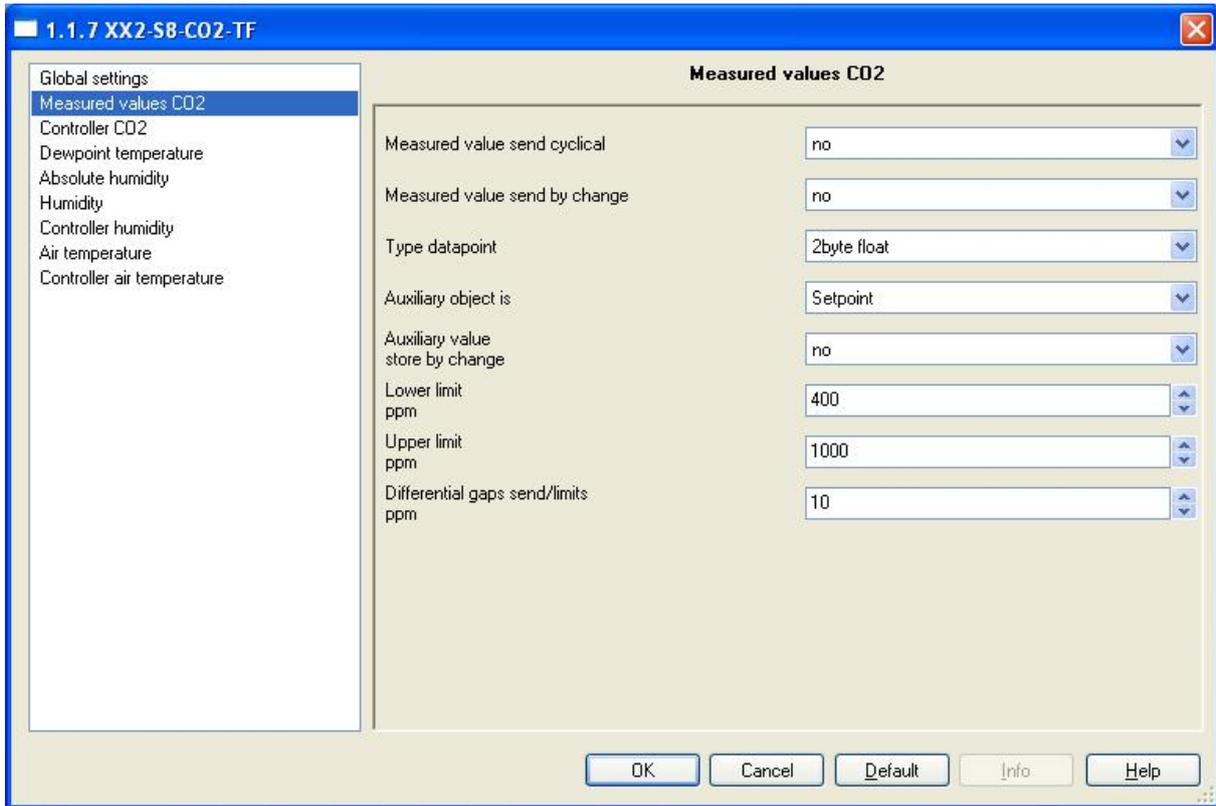
**Save Auxiliary Quantity when change occurs: Yes/No** When the auxiliary quantity is changed the new value is carried over to EEPROM and saved in case of a bus voltage breakdown. This should be used only when the set point is not frequently changed as EEPROM has only a limited memory cycle.
