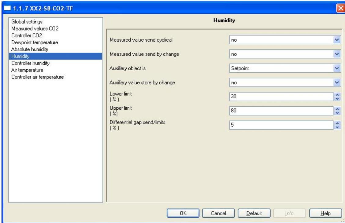
The settings for the arithmetic value of the air humidity are analogue for the measured value of CO2. The rates for thresholds and hysteresis should be done in steps of 1%.
