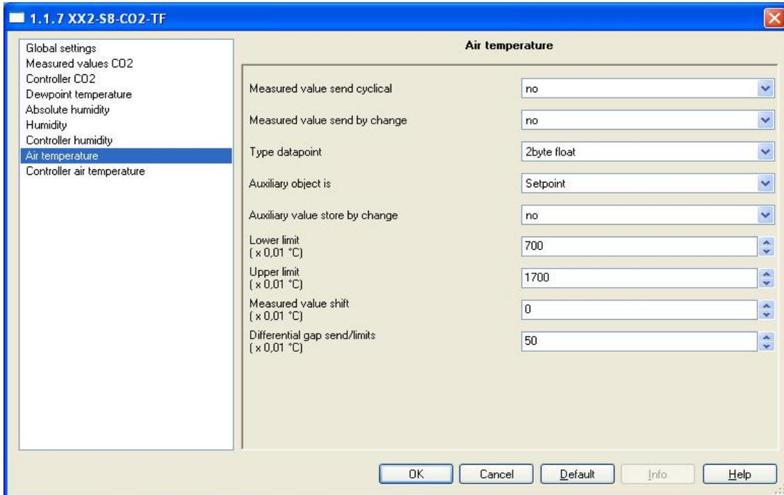
The settings for the measured value of air temperature are analogue for the measured value CO2. The rates for the thresholds and hysteresis should be done in steps of 0,01°.
