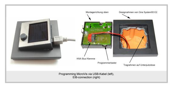
The -cable is stuck from underneath directly on to the circuit board with an KNX-clamp. The display can then be clicked into the box with the suitable single frame. To connect the USB-cable, pull the display lightly out of the socket from the upper side. It is not necessary to interrupt the KNX-connection.
