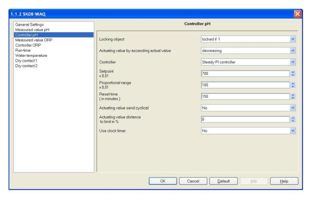
Actuating value by ascending actual value: decrease/increase The Actuating direction of the controller can be adapted to the characteristics of the controlled system.
