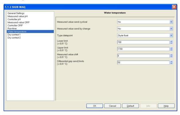
All settings for the rider "Water temperature" should be made analogous to "Measured Value pH" The threshold and differential gap can be set in the range of  $0^{\circ}$  to  $100^{\circ}$ C in steps of  $0.01^{\circ}$ .
