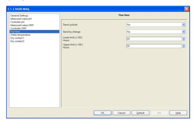
The operating time of the sensor pH/ORP is important for controlling the calibration of the electrodes. The current operating time can be set for either periodic or hourly output. Thresholds can be configured as alerts for recalibration. Calibration times vary according to the type of electrode and the manufacturer. The usual time period is between 3 and 6 months (2000 – 4000 hours).
