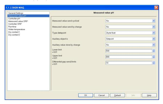
Auxiliary object is: Set point/Upper Threshold/Lower Threshold Every controller has an auxiliary quantity which can control either the set point of the controller or the limit values.
