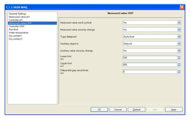
All settings for the rider "Measured Value ORP" should be made analogous to "Measured Value pH" The threshold and differential gap should be set in the range of -1200 to +1200.
