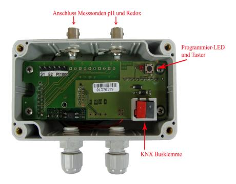
The electrodes must be checked and calibrated at regular intervals. Should deviations occur more frequently and the time it takes the display to show a data change becomes longer, the sensors should be changed.
