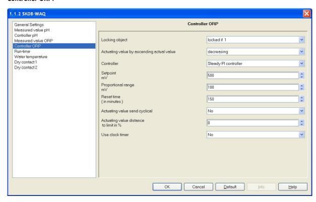
All settings for "Controller ORP" should be made analogous to "Controller pH". The set point, differential gap and proportional area should be set in the range of -1200 to +1200.
