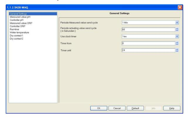
When using the **internal timer**, there are two additional objects for the system-time and –date available. Each controller can be locked independent from each other depending on the time. In this page you can set whether the timer is used at all and the span of time the controllers are active. Whether the timer is used for a controller is determined at his parameter page.
