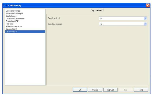
The Parameters "Send on change" and "Send periodically" can be set independent for the 2 dry contact inputs.
