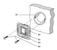
Figure 2: Mounting the bus coupling unit UP 114/02
