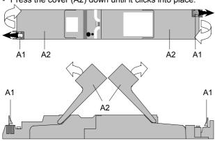
Figure 2: Opening and closing the cover lids
