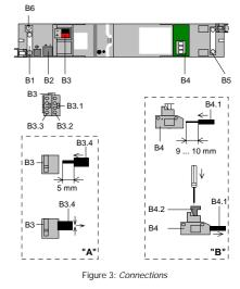
Connecting receiver cable (Figure 3 " B")
