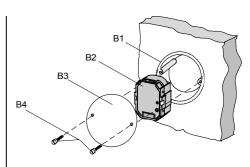
Figure 2: Mounting the shutter switch UP 520/11
