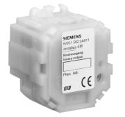
The binary output UP 562/11 is a box mount switching actuator (60 mm Ø, depth 60 mm, a.s.o.). The box mount has to be covered with a universal-cover (ordering separately). Via its 2 outputs it can switch 2 separate groups of electric devices. The load circuits are connected via screwless connection blocks and the EIB bus line is connected via screwless plug-in connection blocks. The binary output UP 562/11 consists of the device (hardware) and its application programs (software).
